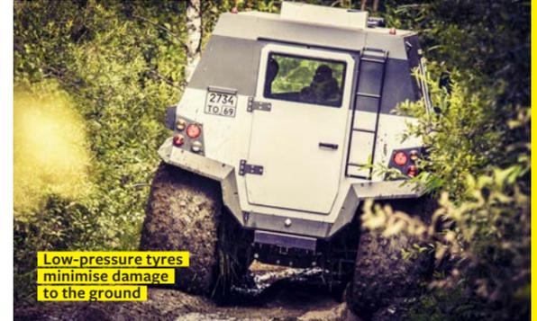
Low-pressure tyres minimise damage to the ground
